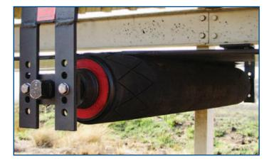
The new tracking technology by TSN can be delivered in virtually all belt widths and eventually produced according to the customers' wishes. The Tru-Trac tracking roller is delivered with a warm vulcanized rubber running surface. The two-bearing construction guarantees an optimal sealing. To this day no existing tracking roller can compare to the Tru-Trac tracking roller. Your belts are sure to run in a straight line.
