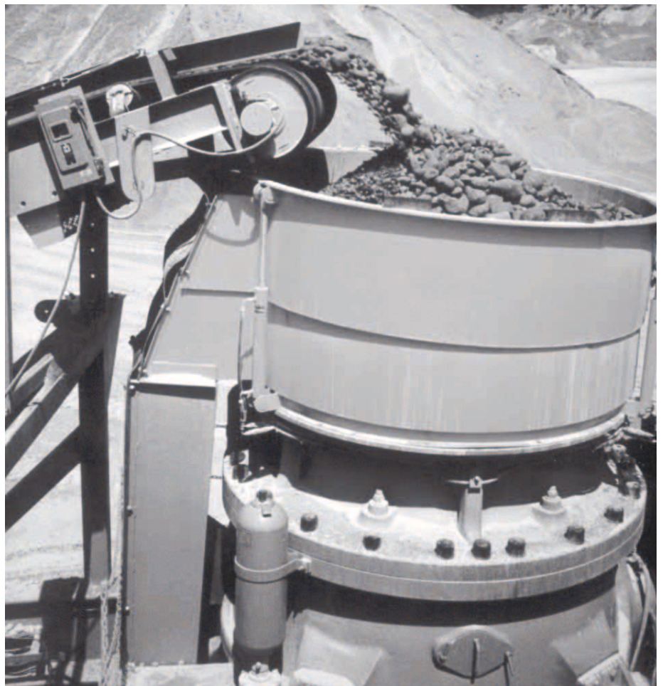
Crushing & Screening. A motorized pulley in its right element!
